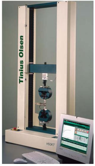
Fig. (3-2) Tensile test machine
