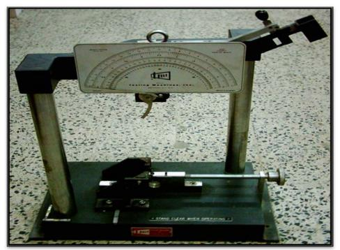
Fig.(3-6): Charpy impact test instrument
