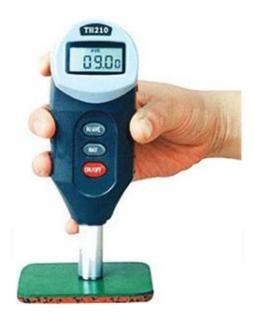
Fig. (3-7): Durometer Hardness instrument from type (Shore D)
