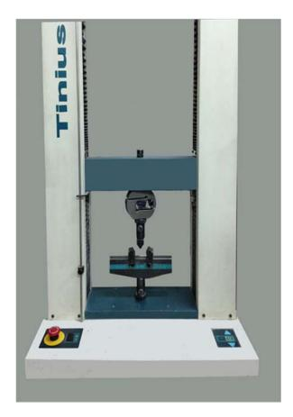
Fig. (3-4) Flexural test machine
